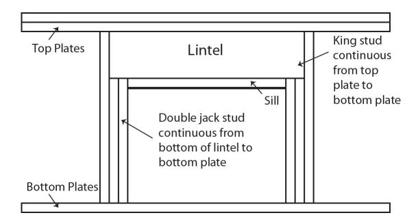
WOOD LINTELS / HEADERS – supporting roof and ceiling loads with a max. truss length of 32'
