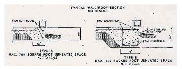
When placing reinforcing steel, all laps in steel shall be 30 times the diameter of the steel used; i.e., 10 metre bars (1/2 inch) = 15 inches lap; 20 metre bars (3/4 inch) = 22 1/2 inches lap.
